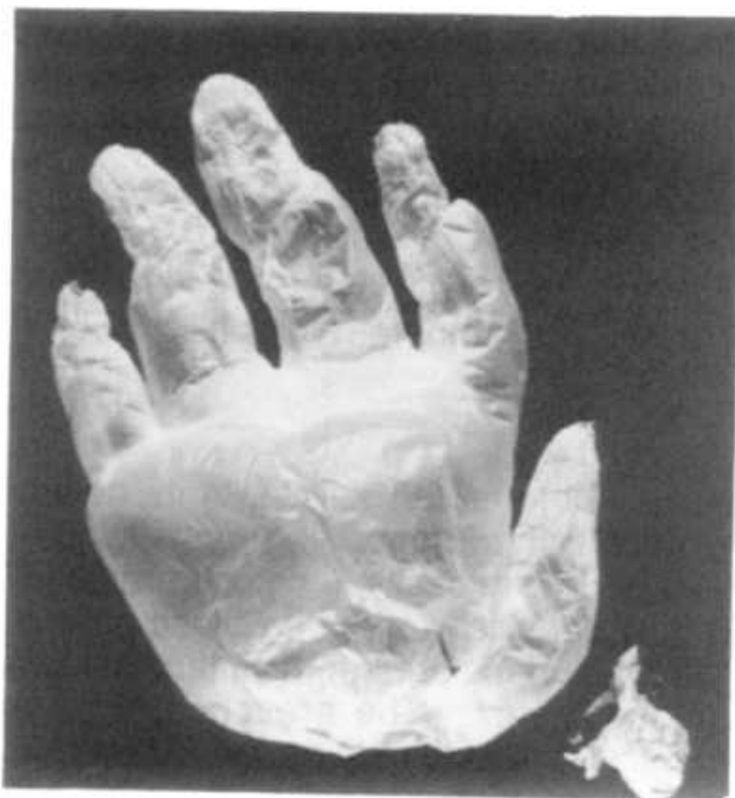
Fig. 3. Dried Acetobacter cellulose formed into a seamless glove shape in situ during cellulose biosynthesis.
